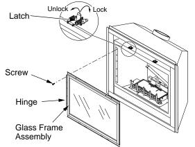
Figure 42 - Removing/Replacing Glass Door
